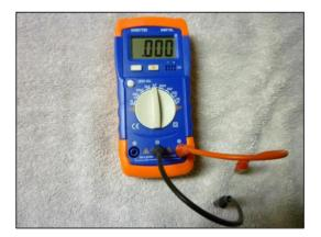
A Honeytek A6013L Capacitor Tester (called a condenser in automotive jargon) is available through Amazon for about \$22. The tester will tell you not only if the condenser is good or bad, but the actual value in micro-farads. Set the pointer on two micro farads.
