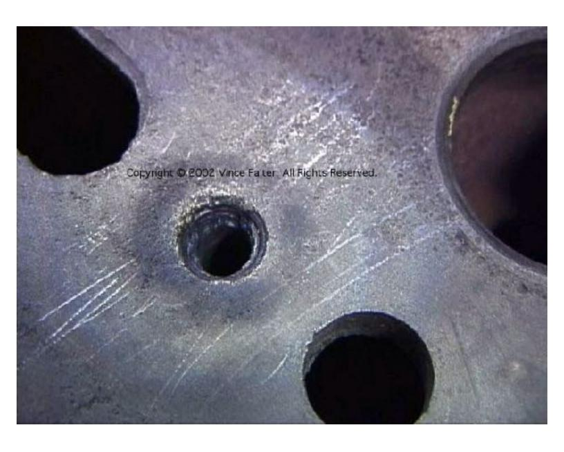
Just place the washer over it and carefully fill the upper portion of the hole first, then TIG weld out to the washer.
