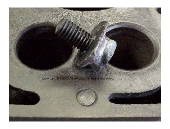
**Here is a beginning and an end:** A flush broken stud in the block and a formerly flush broken stud which had a flat washer and hex nut TIG welded to it. It was then soaked with Aero Kroil Penetrating Oil while hot, and backed out on the low setting of an impact gun.
