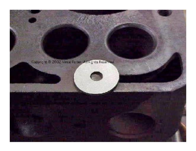
TIG weld the washer to the stud. I prefer to start the arc on the stud and work my way outward in a spiral while adding filler. After welding, spray liberally with Kroil and try to get it under the washer.
