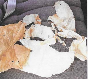
and then remove the gas gauge – low and behold - looking in the gas gauge hole - there WAS my "out of GAS" stopping problem. The spray on gas tank coating(liner) was in a clump at the bottom of the gas tank.
