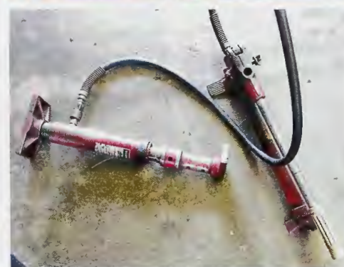
A Hydraulic Power unit is used to push the frame back into position.
