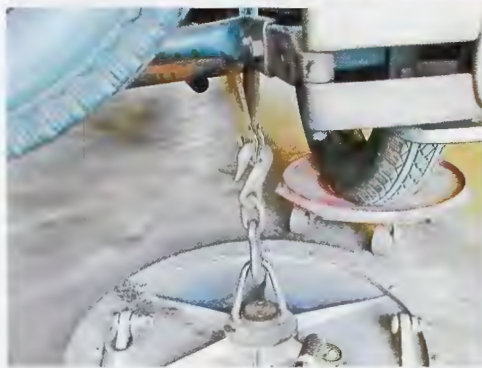
Above - In the rear I use a suction machine to grab the floor. This operates on compressed air. A Chain and strap are used to grab the car in the rear bumper brace area.
