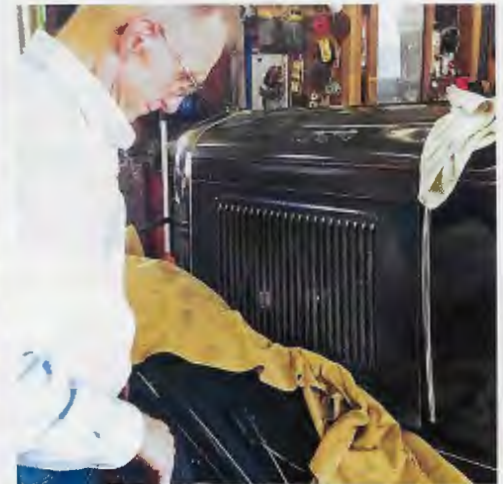
When it starts to get straight the alignment on the hood line will be very evident.
