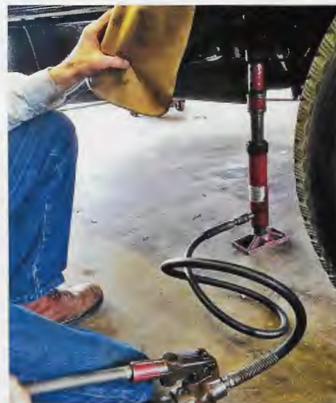
Above - In the rear I use a suction machine to grab the floor. This operates on compressed air. A Chain and strap are used to grab the car in the rear bumper brace area.
