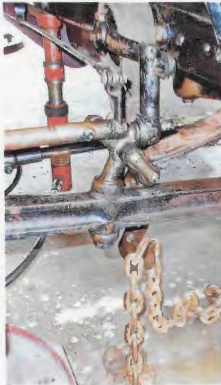
Photos at left and above. The frame is tied down in the front by a strap going over the shock and chained to the floor. I have a tie down anchor in the concrete floor for accomplishing this.
