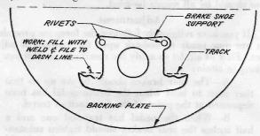
This track must be straight and smooth or all the fiddling in the world will not provide good brakes. To accomplish this task the track will have to be removed from the backing plate by removal of rivets. The track should then be built up with weld and ground to a straight surface. This operation is essential.
